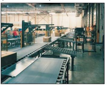
loop of minimum-pressure accumulation conveyor. The cartons then travel through a scanning location where their dock destination is determined. The information is transferred to the system's primary logic controller which activates an overhead pusher at the appropriate dock location. Cartons flow onto an extendible conveyor that transports them into trailers for loading.
